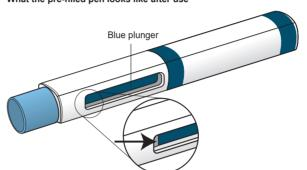
The blue plunger gradually slides down the viewing window during the injection.
