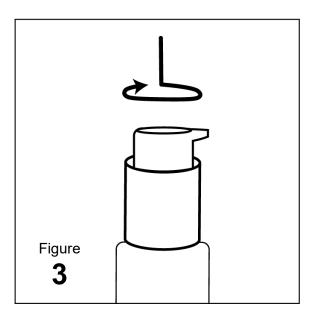
4. Twist the dosage pump into open position. See Figure 4.
