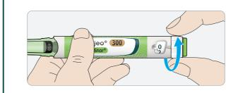
How to read the dose window Even numbers are shown in line with the dose pointer:
