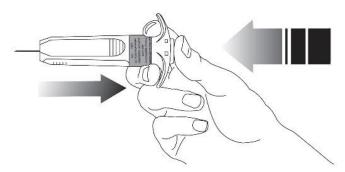
12. Then release the pressure on the plunger. The needle will automatically retract into the needle guard where it will be locked permanently.
