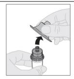
10. Connect the solvent syringe to the vial adapter by inserting the tip of the syringe into the adapter opening. Firmly push and turn the syringe clockwise until it is securely connected.
