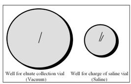
Needles protruding from these two wells accommodate supplied sterile eluant charge vials and sterile eluate collection vials. The eluting solvent consist of 5ml or 15ml Sodium Chloride 0.9% solution, in prepacked septum-sealed vials.
