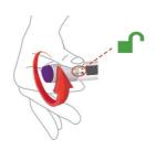
Unlock by turning the lock ring.
