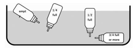
The approximate quantity of liquid in the canister is indicated by the position of the canister in the water.
