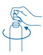
Mounting the dosing pump on the bottle:
